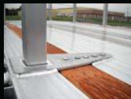
Deck Pockets Along Side Rail
