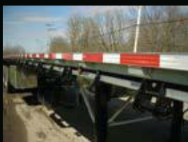
Western Side Rail with Fixed Angle Winches and Fixed Strap Hooks
