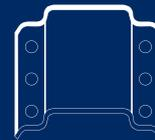
Attached to the extruded aluminum floor, the 80,000 psi high strength steel hat-shaped top flange provides additional lateral stability to the trailer.
